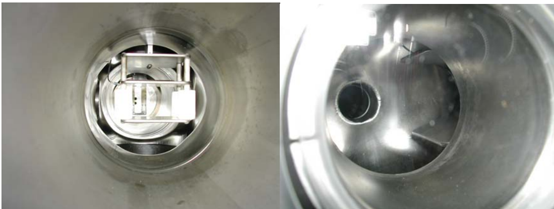
Figure 3. Pictures of sweep plates from inside (left) and outside (right) the Helicon.
